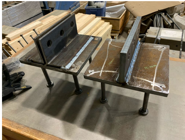
Figure 1.1 – Typical four-stud embedded plate with a double angle shear connection (left) and a shear tab (right) for connecting to the web of a wide-flange beam or channel.
