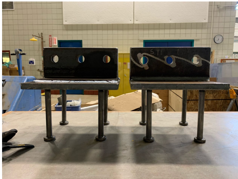
Figure 2.1 – Headed studs welded to a steel plate
